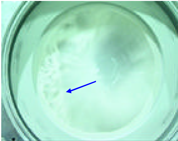
[Fig. 10a] Counter impulse method with dry product during the gas impulse.
