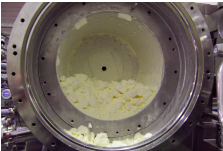
[Fig. 11b] Agglomeration after fixed bed drying. The product is still wet within the lumps.
