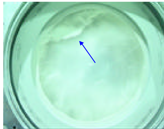
[Fig. 10b] Counter impulse method with dry product shortly after the gas impulse - the cake remains
