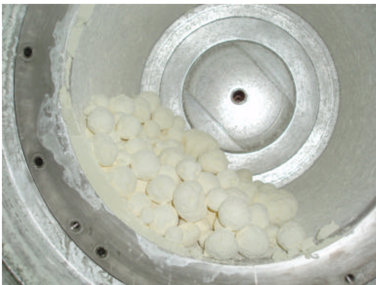
[Fig. 13] Product discharge after conventional fluid bed drying with a product tending to agglomerate. The filter drum is covered with incrustations of the product.
