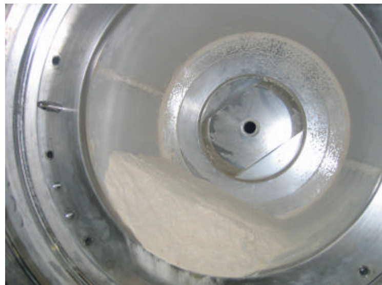
[Fig. 12b] Dry powder, ready to be discharged with no residual heel cake. The counter pulse method avoids caking of the filter drum.
